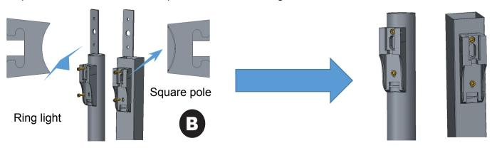
Step3: Fix the lamp body with the bracket installed to the bracket B of the pole and fix it with M4 screws. (Figure C)
